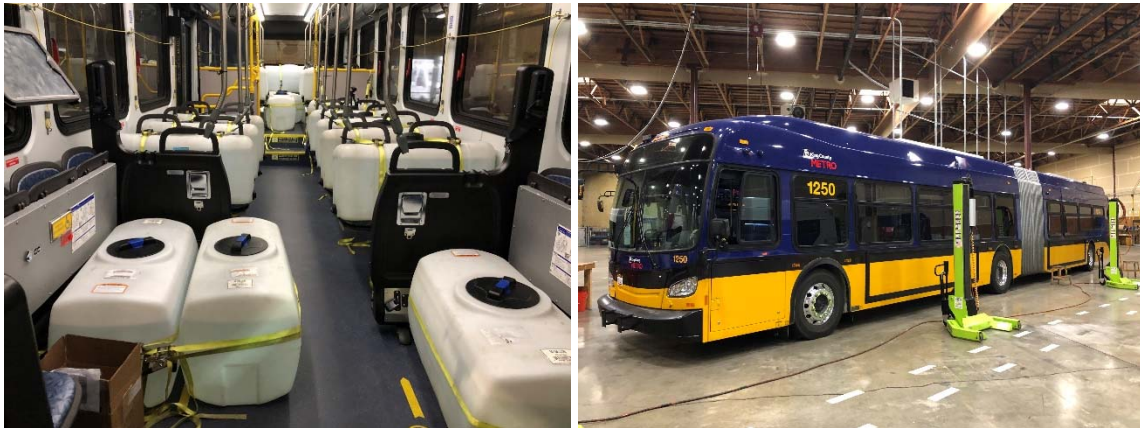
Left to right: A Proterra battery-electric bus with onboard water to simulate passenger loads; A New Flyer battery-electric articulated bus.
