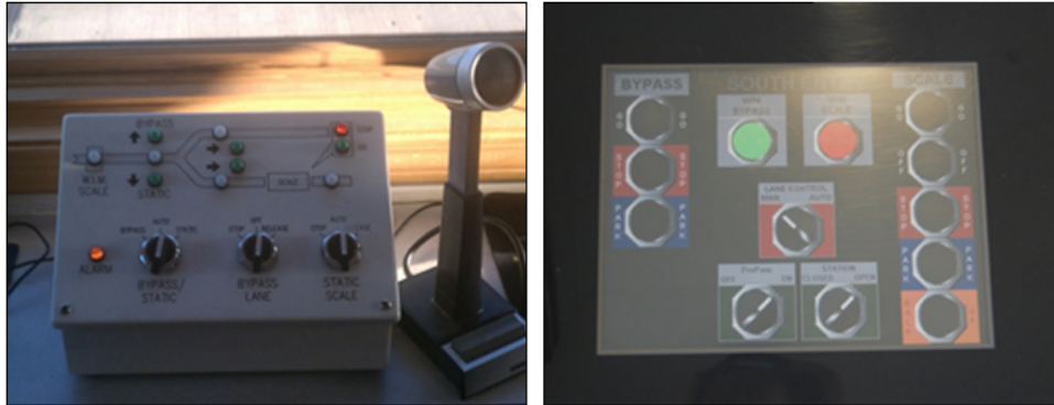
Figure 2.12 Manual and Electronic Inspection Station Signaling System Controls
