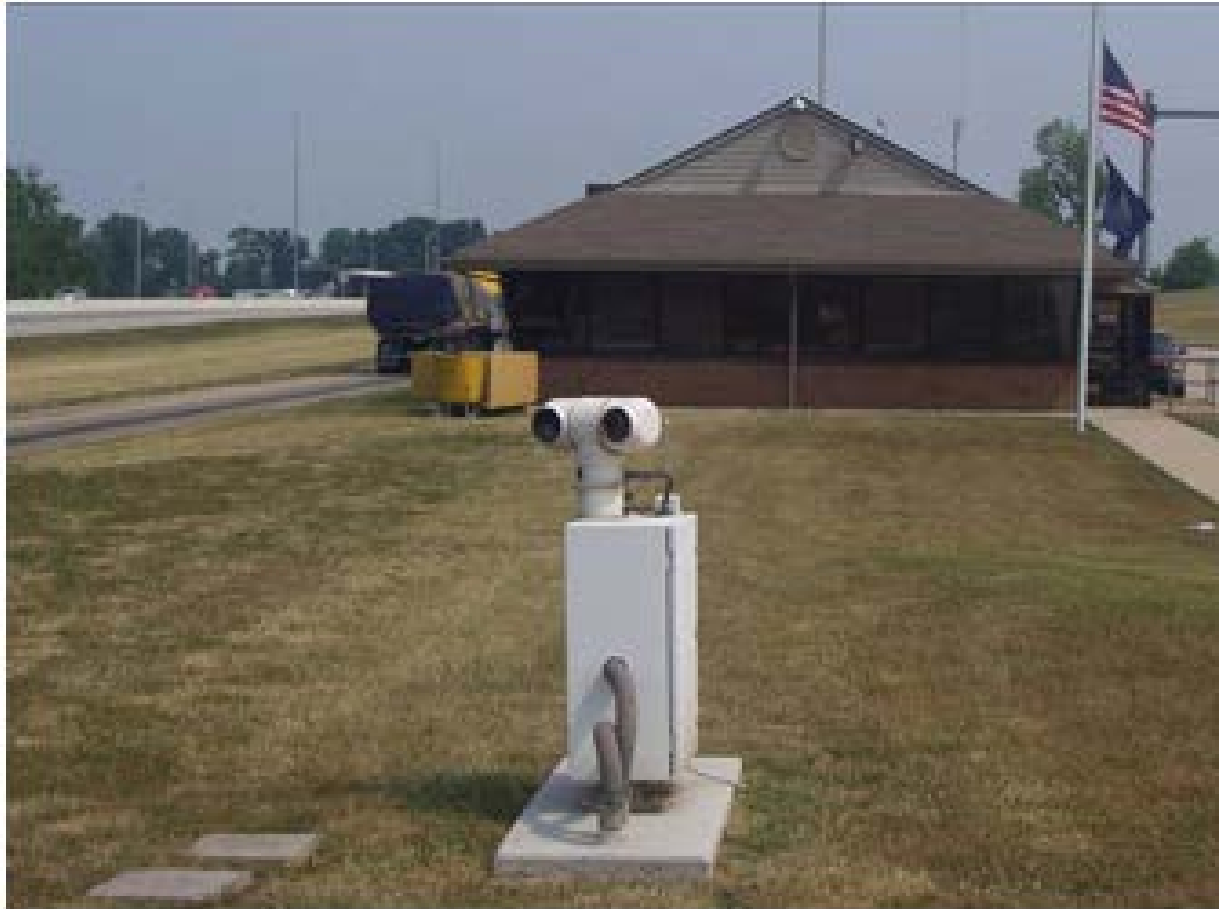
Figure E.11 Thermal Inspection Device with Full Color and Thermal/ Infrared Camera – Kentucky
