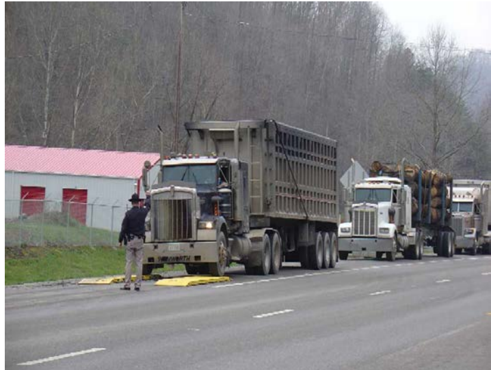
Portable Scales in use on U.S. 23 in Floyd County, KY.
